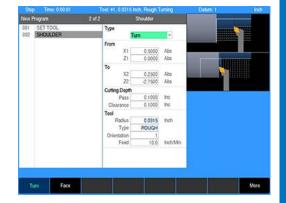
A contour's profile is defined by one or more connected lines, arcs, blends, or chamfers. For this example, the contour consists of a single arc.
