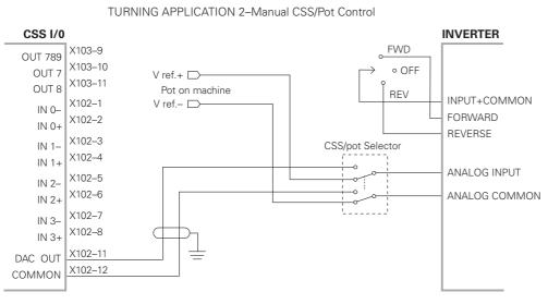
Example of switching to manual spindle speed control
