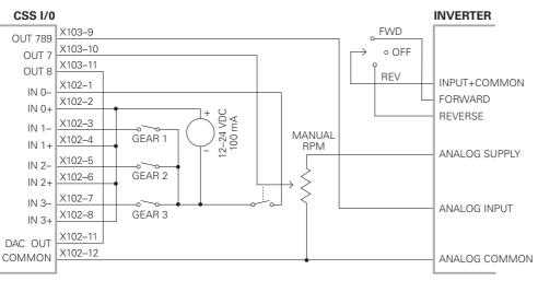
Example of gear detection and switching to manual spindle speed control
