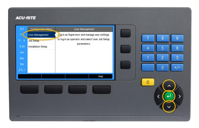
Use the up and down arrow keys to highlight the Supervisor Login menu, then press enter.
