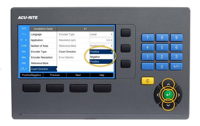
Press the left arrow key three times to get back to the DRO screen. Repeat this sequence for additional encoders as needed.
