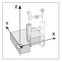
The position of the tool at any given moment is called the Actual Position I, while the position that the tool is to move to is called the Nominal Position S. The distance from the nominal position to the actual position is called the Distance-To-Go  $\mathbf{R}$ .
