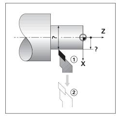
To set a tool offset using Lock Axis:
