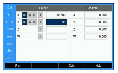
The coordinates are entered as absolute dimensions; the datum is the workpiece zero. Using this figure example:
