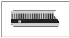
Encoders that have one or more marks on fixed intervals have to re-establish the datums correctly. It is necessary to use the same exact reference mark, during the Reference Mark Evaluation routine, that was used when the datum was first established.
