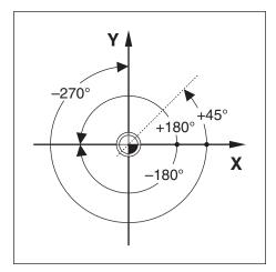
The Zero Angle Reference Axis is the 0.0° position. It is defined as one of the two axes in the plane of rotation. The following table defines the Zero Angle where the position of the angle is zero for the three possible planes of rotation.
