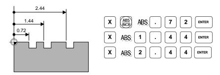
When you enter an incremental preset, the tool **must** be positioned at the location you are dimensioning from.
