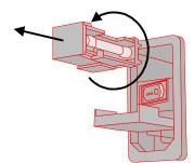
3. Remove the fuse, move the shorting bar to the other side, install the proper fuse, and push the block back into place.
