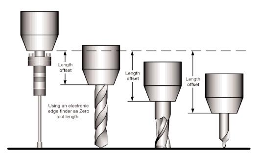
If you begin setting the tool length offsets by setting Datum using an electronic edge finder it must have a fixed and repeatable length. The current tool information cannot have a length value. All of the tool length offsets in the program will be the difference in length between the tool and the edge finder.
