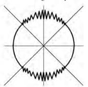
Stick-Slip of an axis, esp. at low speeds (in this case, Y-axis)
