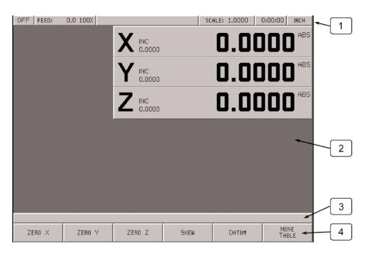
Status bar - displays the servo motor status (ON/OFF), feed rate, current tool, scale, job clock, and the current display setting (inches or millimeters).
