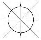
Axis Reversal Spike shows an axis sticking when velocity reaches zero (in this case, Y-axis)
