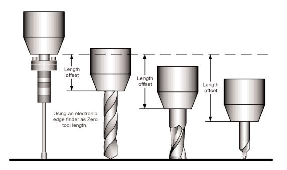
All tool lengths originate from datum. There are several different ways to establish datum, such as "touching off" with an empty spindle, using a repeatable standard or using an electronic edge finder (refer to **Establishing Datum**).
