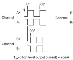
$I_{OH}$  = (High level output current) = 20mA V<sub>OH</sub> = (High level output voltage) < 2.5Vdc
