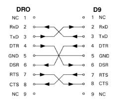
Pin connection for serial port with handshaking.
