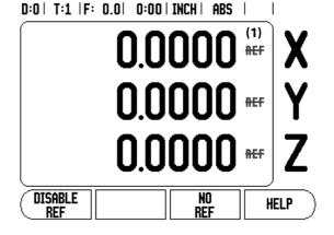
The 200S can still cross over reference marks at a later time. Such as if it becomes necessary to define a datum that can be re-established after a power interruption.
