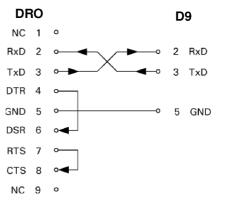
Pin connection for serial port without handshaking.
