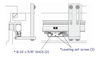
Insert the two \*8-32 x 5/8" SHCS. Ensure the bracket assembly is adjusted to provide proper screw head clearance. **Do Not** Tighten Screws at this time.
