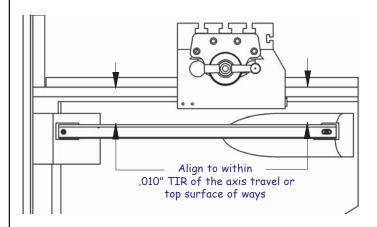
Align the spar top and front surface to the axis travel.
