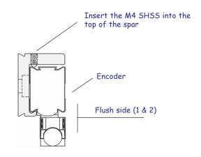
Insert the encoder into the spar as shown, and center from end to end. Tighten the center set screw only.
