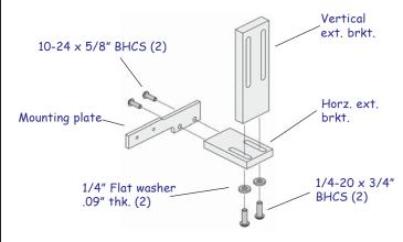
Assemble the brackets, fully extending the horizontal extension plate.
