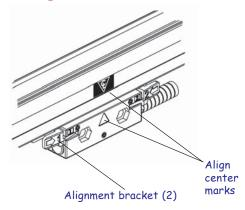
Slide the reading head and brackets along the scale case until the center marks on the scale case and reading head are aligned.
