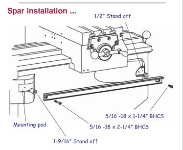
Attach the spar to the knee with the standoffs onto the mounting pads.
