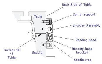
• These instructions will guide you through installing the encoder as shown in this view.
