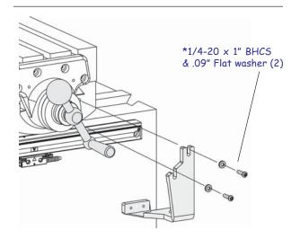
• Attach the bracket to the saddle.
