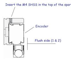
• Insert the encoder into the spar as shown, and center from end to end. Tighten the center set screw only.
