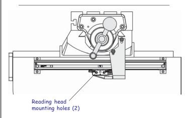
Adjust the bracket so that the reading head mounting holes align with the reading head casting. Secure the bracket in place.
