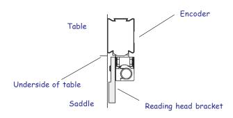
With the table at its center of travel, set the encoder against the table and the reading head bracket against the saddle.
