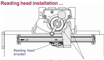
Transfer punch mounting slot locations to the end of the saddle
