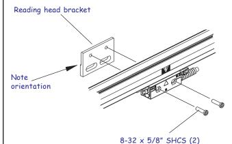
Temporarily attach the bracket to the reading head.
