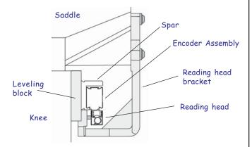
• These instructions will guide you through installing the encoder as shown in this view.
