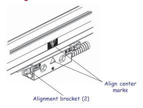
Slide the reading head and brackets along the scale case until the center marks on the scale case and reading head are aligned.
