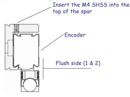
• Insert the encoder into the spar as shown, and center from end to end. Tighten the center set screw only.
