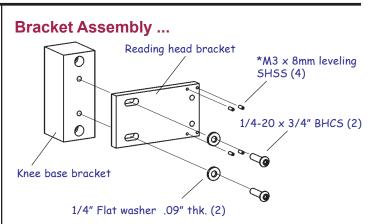
• Assemble the brackets loosely for future adjustment. Insert the leveling screws flush with the bracket surface.
