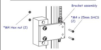
• Attach the reading head bracket assembly to the reading head.
