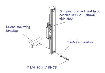
Attach the lower mounting bracket to the encoder as shown. Encoder has the numbers 1 & 2 facing out.
