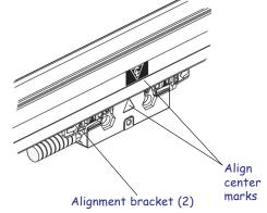
• Slide the reading head and brackets along the scale case until the center marks on the scale case and reading head are aligned.
