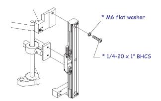
• Attach the encoder assembly to the upper bracket.
