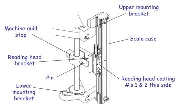
These instructions will guide you through installing • the encoder as shown in this view.
