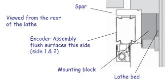
• These instructions will guide you through installing the encoder as shown in this view.
