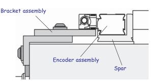
• These instructions will guide you through installing the encoder as shown in this view.
