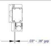
• There will be a gap of .03" - .018" between the bracket assembly and the reading head.
