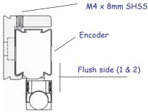
• Insert and center the encoder in the spar from end to end and tighten set screws to secure in place.
