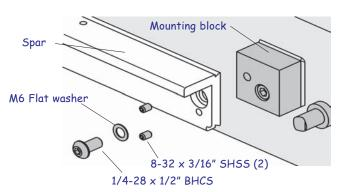
• Insert the two 8-32 x 3/16" SHSS into the spar at each end and attach the spar to the mounting blocks.
