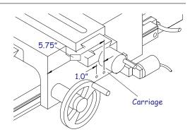
• **Pre 1988 lathes:** Drill and tap hole locations for a 1/4-20 x 1/2" deep. The height of the mounting holes are located by attaching the bracket assembly to the reading head and transfer punch using the bracket.
