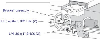
• With the carriage at its center of travel, attach the bracket assembly to the carriage.
