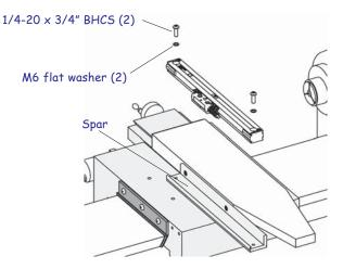
• Insert the encoder into the spar and seat the encoder into the lip of the spar. Secure in place.
