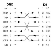
Pin connection for serial port with handshaking.
