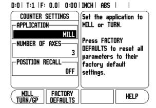
The Position Recall feature, when it is "ON", will store the last position of each axis when power was turned off, and then redisplay that position once power is turned back on.
