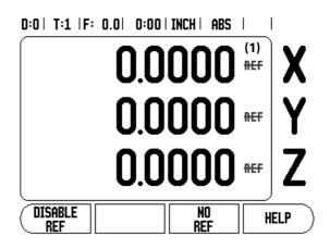
The W550 can still cross over reference marks at a later time. Such as if it becomes necessary to define a datum that can be re-established after a power interruption.
