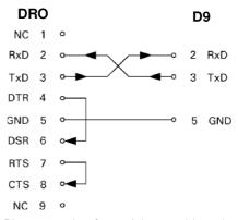
Pin connection for serial port without handshaking.
