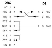
Pin connection for serial port without handshaking.
