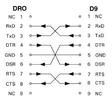
Pin connection for serial port with handshaking.
