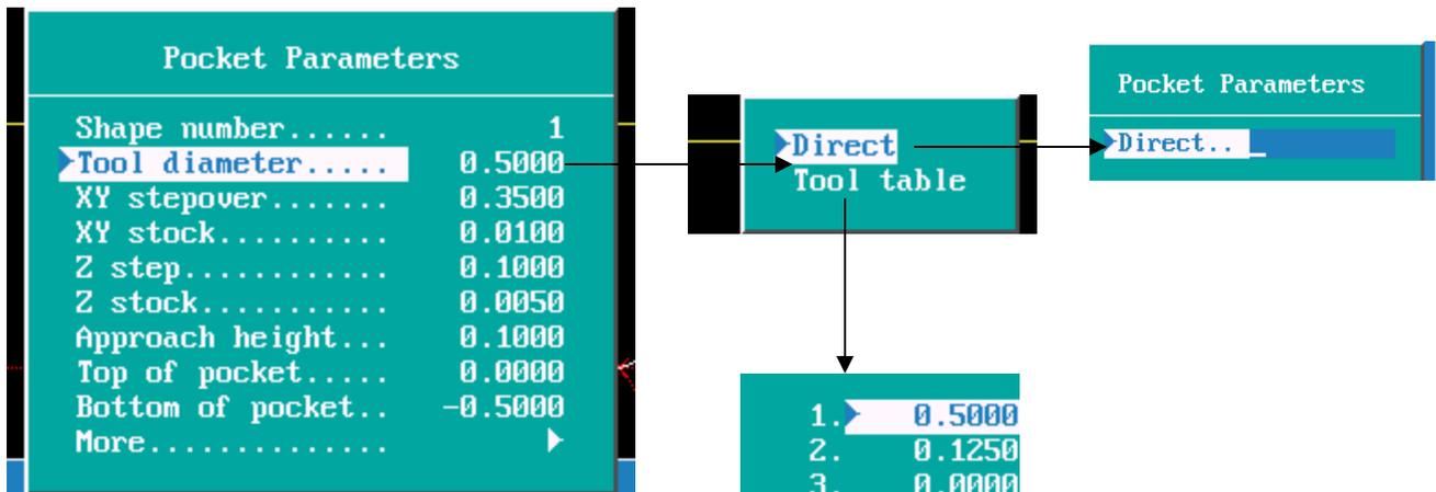
There are two methods of entering tool diameters, direct just type in value and select it from toll table.
