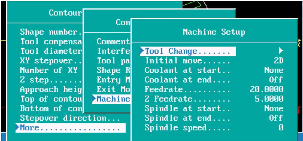
Note: Coolant and spindle at start are entered as **None** and turned **Off** at end, as they are still on from pocketing.
