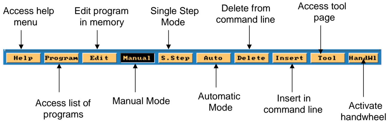
**Note:**When handwheel is active colors will be reversed in box as shown below.
