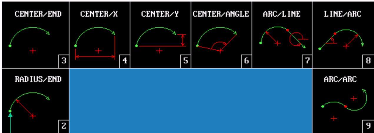
Tool must be at start point before inputting arc's
