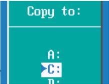
With C: High lighted Press
