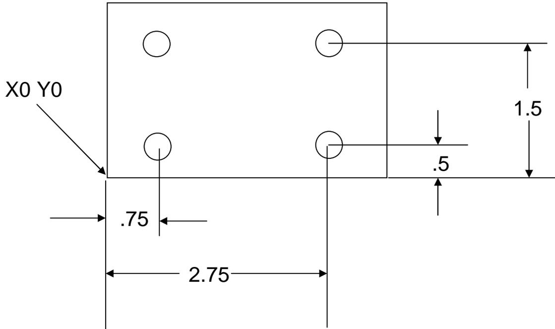
This part needs to have 4 hole drilled .25 dia and .5 deep
