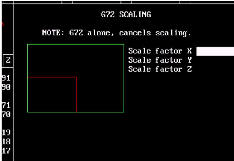
When using scaling if there are any the axis must be scaled the same on both of these axis. If part is required to be half size .5 would be factor. G72 alone will turn off scaling.
