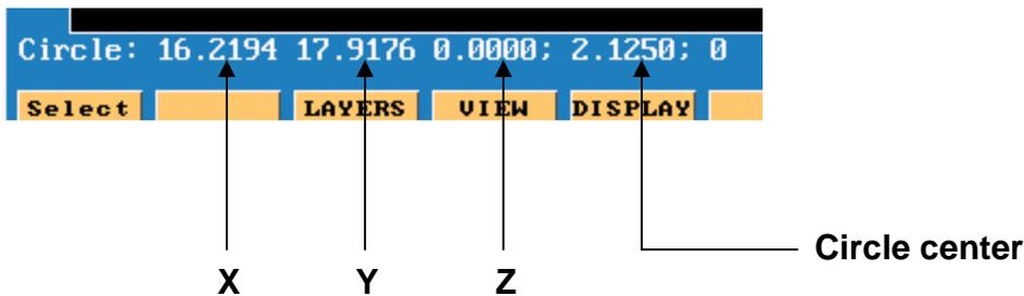
Now press **ALT** key and letter **T** at the same time. This will in put these coordinates in to the **SETUP** and change **X0 Y0** to the center of hole.
