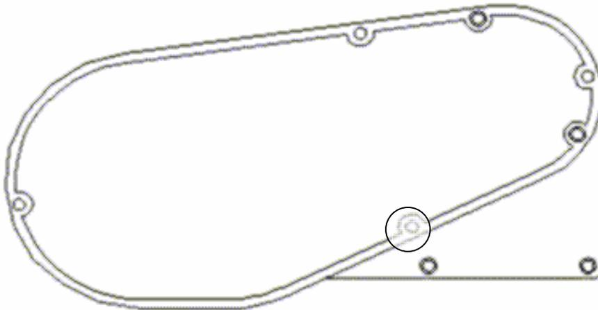
The circled area is blown up below. It shows an error in the drawing, where two lines are not connected. It will stop, select next element and the following message will appear.
