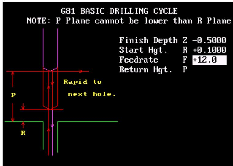
Enter values Finish Depth -.5 press down arrow, enter Start Hgt. .1 down arrow and Feedrate 12
