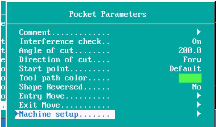
Angle of cut can be left at default or an angle entered, on this part an angle of 200 deg's will be entered.
