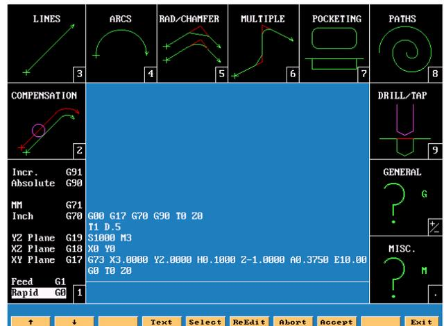
**Note:** The center of the screen. There are two different displays, one has text about **Help** the other shows the program as it is being entered.
