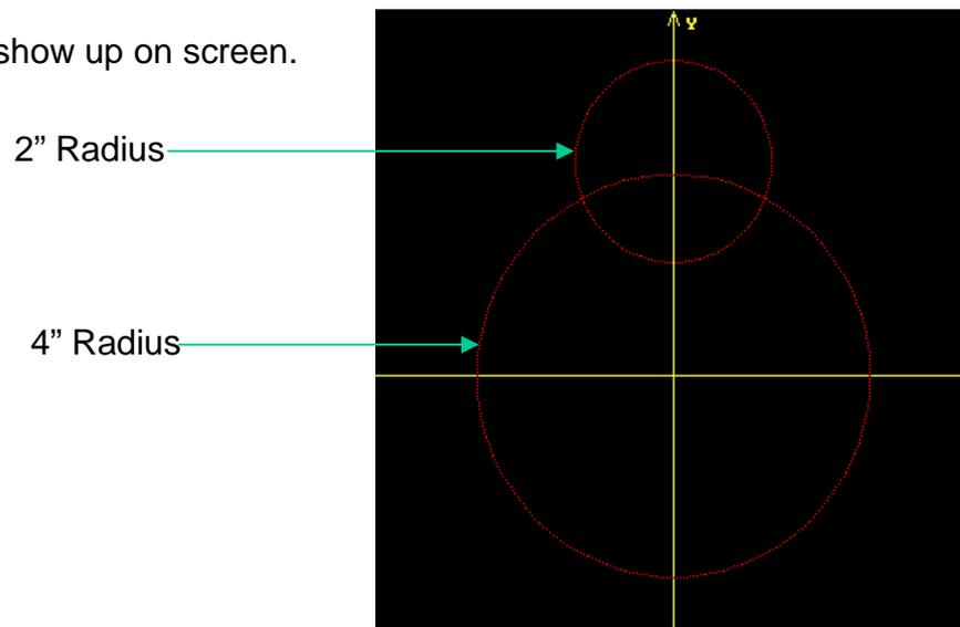
The next geometry required are two points at the intersect of the 4" radius circle and the -3.75 line. To do this use icon circled below.
