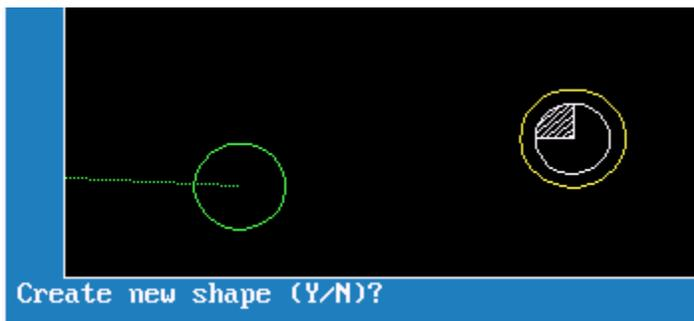
The green circle is the last of previously selected holes. The yellow circle is the one selected with right mouse button and in the bottom left it is asking if this is a new shape, the answer is **Y** .It will put a number 2 next to this hole, meaning this is shape 2.
