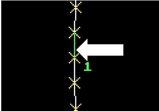
Press **F1** **Select** point mouse arrow to lower end of a line as shown and press left mouse key. Line will turn green as above and put a number at low end of line, the position of the number is the start point. Now point to the line below it and press left mouse key, all of the line will be come green.
