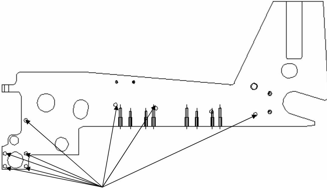
Press **F1** **Select** and pick all holes that are the same size , in this case 8. When going to second set of holes press right key on mouse.
