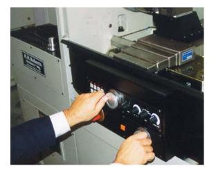
The 4200T has a conversational programming utility. You don't have to have any prior programming experience. Screens are icon-based and you are prompted for data input. The intuitive interaction makes the control easy to learn.
