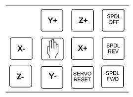
Figure 3-4, Manual Operation Keys
