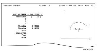
Figure 4-14, ARC (CENTER – END POINT) Graphic Menu
