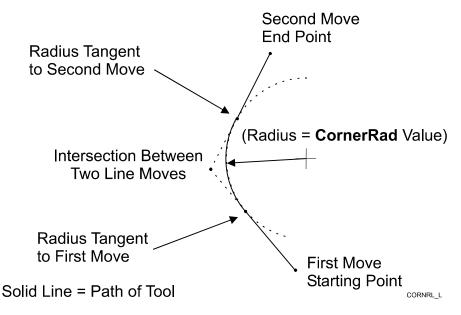
Figure 1-14, Line-to-Line Corner Rounding
