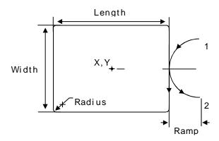
Figure 5-13, Outside Profile Ramp Moves
