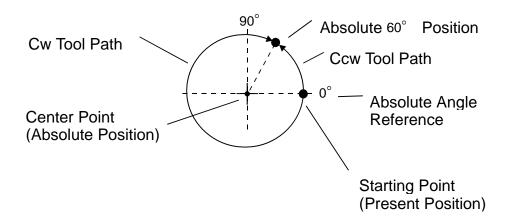
Figure 4-16, Absolute Mode, Center - Angle Arc
