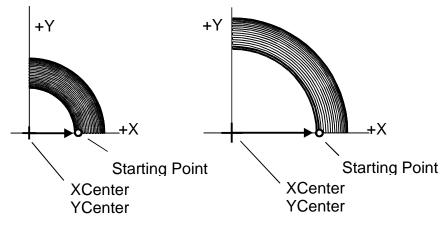
Figure 5-44, Starting Point and Effect on Size
