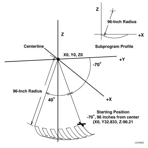
Figure 5-35, Large Radius Mold Rotation
