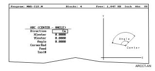
Figure 4-18, Arc (Center - Angle) Graphic Menu
