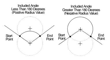
Figure 4-12, Endpoint Radius Arc Types
