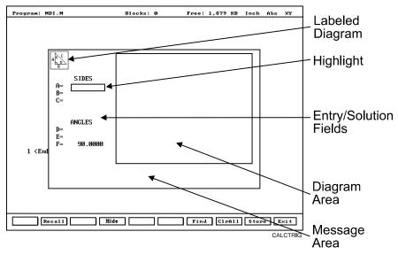
Figure 12-3, Right Triangle Calculator Screen
