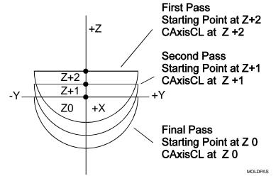
Figure 5-33, Cutting a Cavity Using More than One Pass
