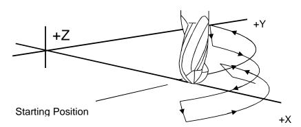
CW Execution Of Moves For Elbow Cavity
