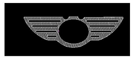
Figure 15-7, DXF Pockets with Islands Completed Example Workpiece
