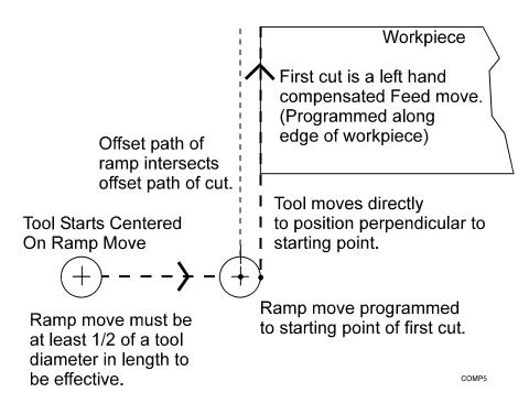
Figure 1-10, Ramping into a Compensated Move
