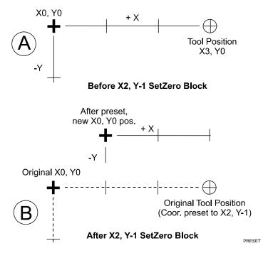
Figure 4-4, Executing a SetZero Block
