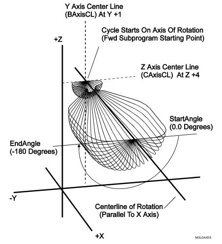
Figure 5-32, Axes of Rotation
