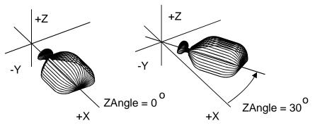
Figure 5-34, Rotating XY Mold Rotations Around Z
