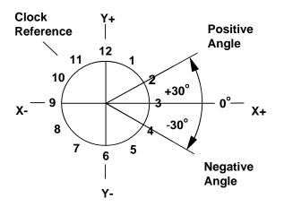
Figure 1-13, Absolute Angle Measurement
