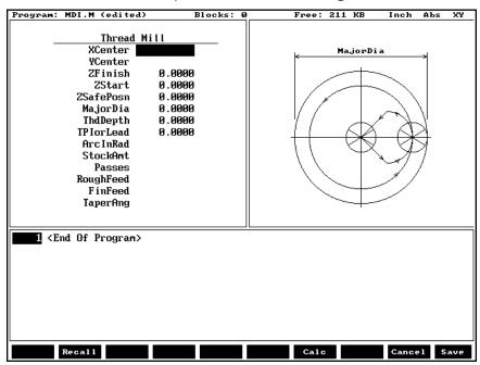
Figure 5-8, Thread Mill Graphic Menu
