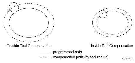
Figure 5-27, Ellipse Tool Compensation
