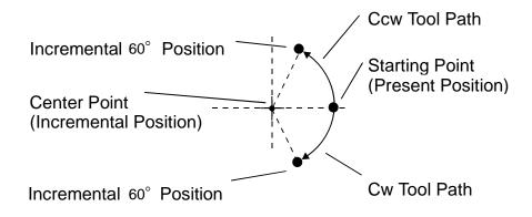
Figure 4-17, Incremental Mode, Center - Angle Arc
