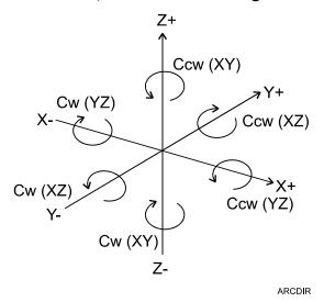
Figure 1-19, Clockwise and Counterclockwise Arc Directions
