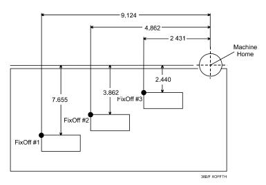
Figure 3-3, Locating Fixture Offsets
