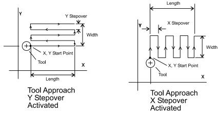
Figure 5-10, Face Cycle Tool Approach
