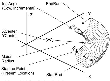
Figure 5-42, Elbow Milling Cycle Details
