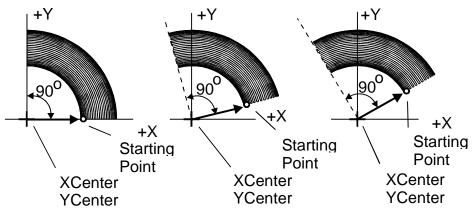
Figure 5-43, Starting Point and Effect on Orientation
