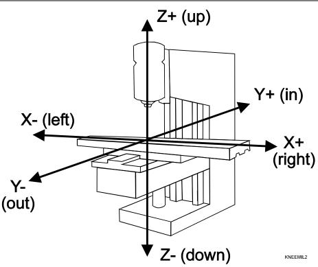
Figure 1-1, Mill Axes of Motion (Tool Motion Orientation)
