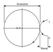
Figure 5-15, Ramp Position for Outside Profile
