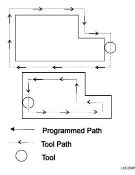
Figure 1-7, Left-Hand Tool Compensation
