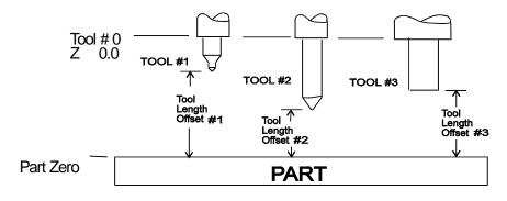
Figure 1-6, Tool-Length Offset
