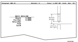
Figure 5-1, BASIC DRILLING Graphic Menu
