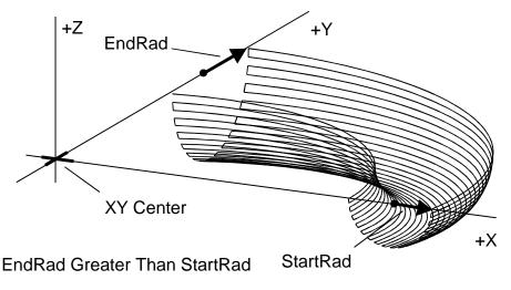
Figure 5-46, Conical Elbow Details
