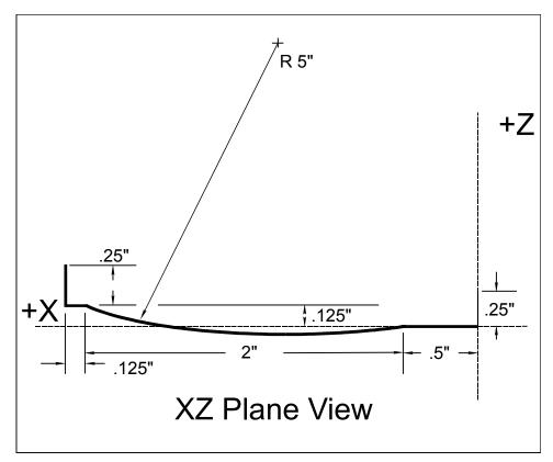
Figure 6-15, Subprogram Layout for Sample Program #9
