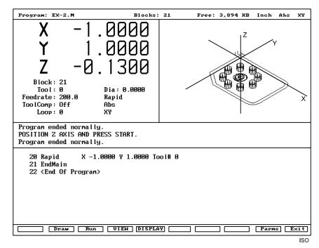
Figure 3-6, Draw Mode (Iso View) Showing Sample Part
