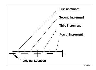
Figure 1-3, Incremental Positioning
