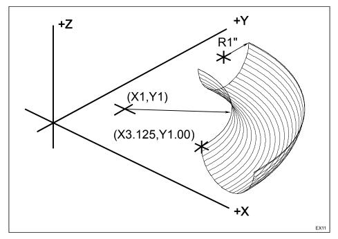
Figure 6-16, Layout for Sample Program #10, Elbow Milling
