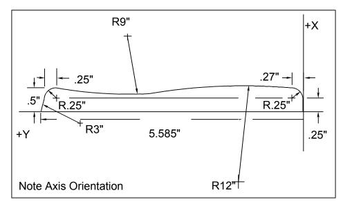
Figure 6-13, Subprogram Layout for Sample Program #8
