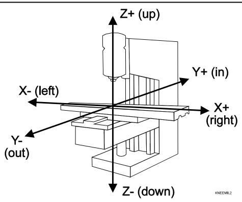
Figure 1-1, Mill Axes of Motion (Tool Motion Orientation)
