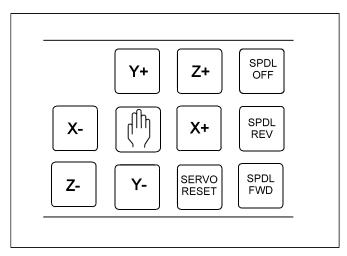
Figure 2-4, Manual Operation Keys
