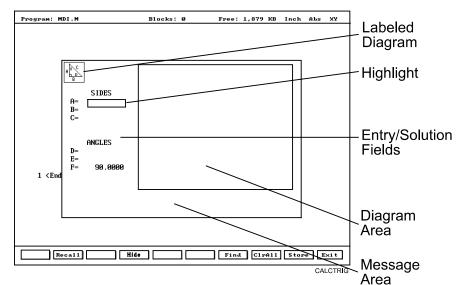
Figure 5-3, Right Triangle Calculator Screen
