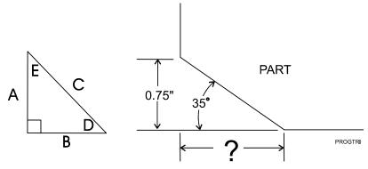
Figure 3-5, Triangle Calculation
