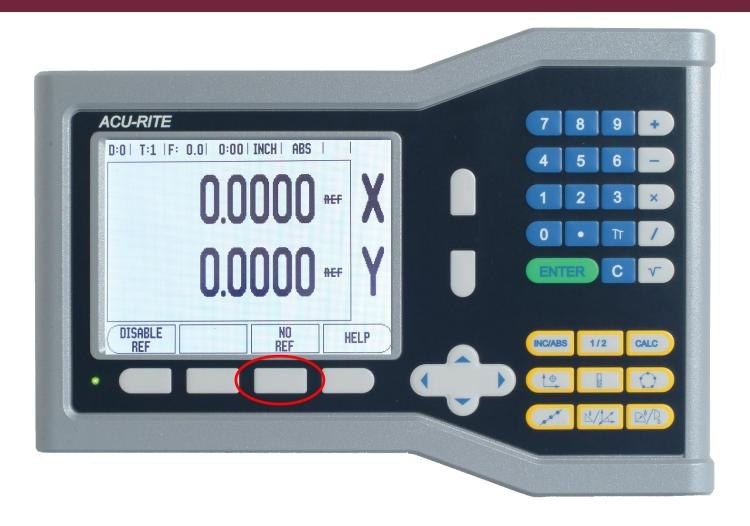
To change the count direction you don't need to reference the scale, so press the "NO REF" soft key.
