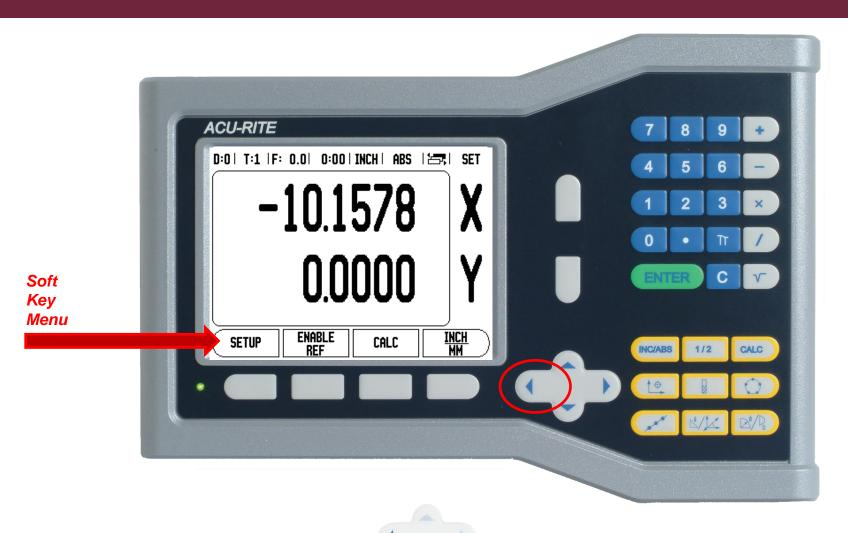
Press the soft key until the first soft key menu space reads "SETUP."
