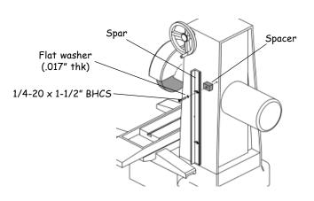
Attach the spar to the column.
