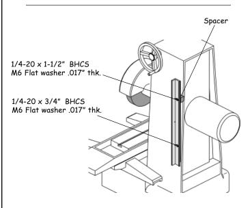
Attach the spar to the column.
