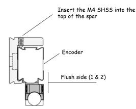
• Insert the encoder into the spar as shown, and center from end to end. Tighten the center set screw only.
