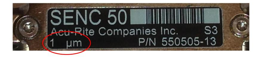
Inspect the reader head ID sticker on your scales. Locate and <u>record</u> the resolution factor on <u>each</u> scale. Each axis may be different —1  $\mu$ m, 2  $\mu$ m, 5  $\mu$ m, 10  $\mu$ m, etc. In this case its 1 $\mu$ m.
