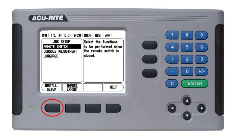
Press the "INSTALL SETUP" soft key.
