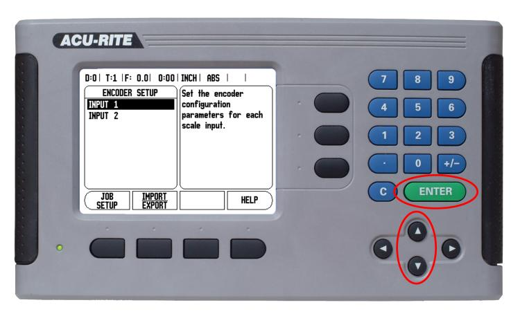
If you need to change more than one axis, highlight the other input axis. Repeat the procedure to change the resolution factor until it matches what is printed on each of the encoders labels.
