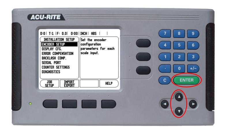
"ENCODER SETUP" should be highlighted. If it isn't, use the or soft keys to highlight it. Then press ENTER
