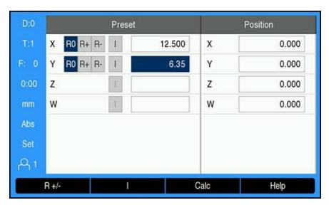
The coordinates are entered as absolute dimensions; the datum is the workpiece zero. Using this figure example:
